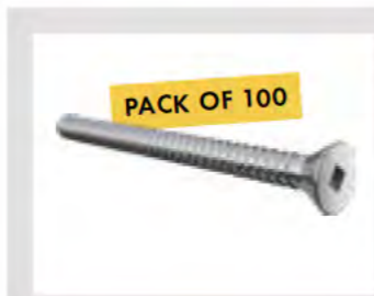
CSK 75mm long square drive Order Code: A50-CSK75-12G • 12G x 75mm long - SS304 • Pack of 100 • Use to affix base plate to posts • If not using welded on base plates
